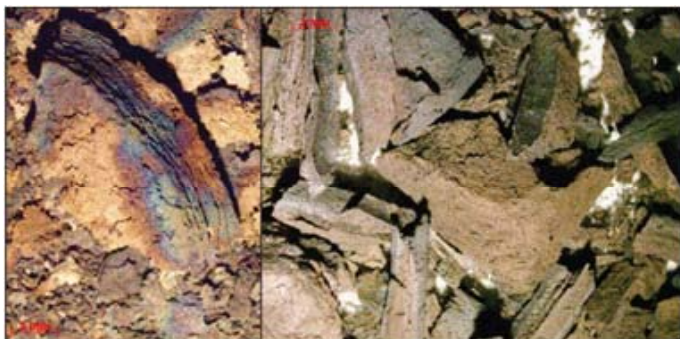
Figure 6 - Sample partially oxidized (right) and a well-passivated sample (left).
